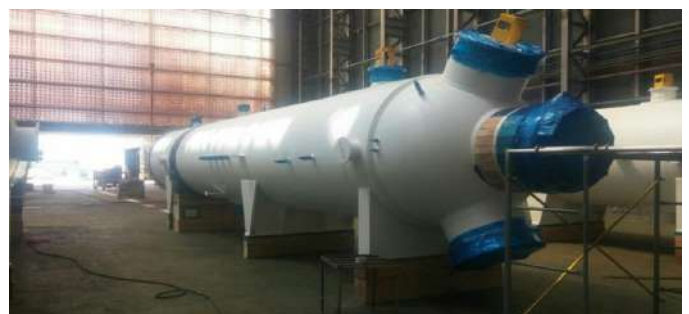
HP Feed Water Heater 8
