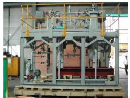
Diesel Oil Filter Package
