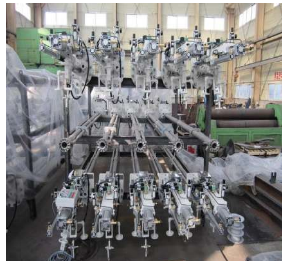
Oil Burner System
