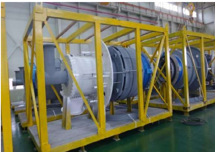
Coal Burner System
